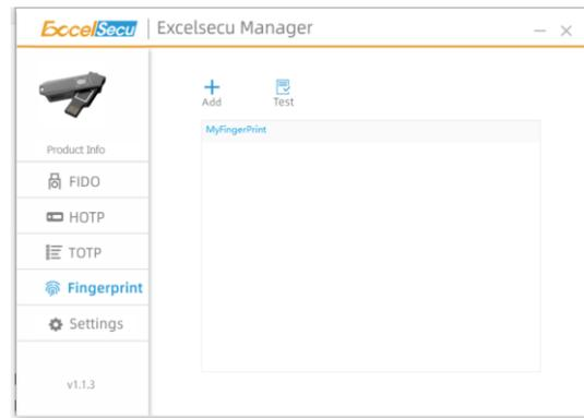
Click **Test** button, the key flashes green light. You are required to verify the fingerprint. For security concern, the key will be blocked if user fails to verify fingerprint 15 times in a row. User can only unlock via reset device (All stored data will be lost).
